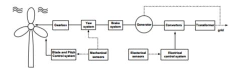
Figure 1. DFIG-based wind turbine structure
